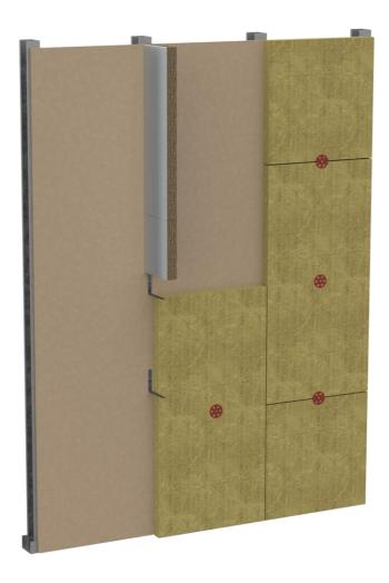
PFC Corofil Cavity Fire Stop CCFS Slabs may be cut and installed horizontally and vertically against an SFS system with calcium silicate cement fibre board and are suitable for cavity widths between 10mm and 600mm.
