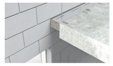
PFC Corofil Cavity Fire Stop CCFS Slabs may be cut and installed horizontally at a slab edge and are suitable for cavity widths between 10mm and 595mm.
