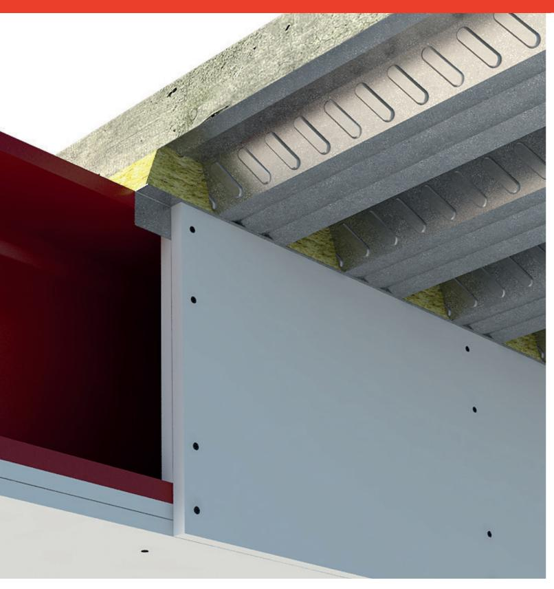
PFC Corofil Linear Gap Seal Block is a stone wool block installed in the trapezoidal profile of a composite profile deck at the head of flexible and rigid wall constructions and above a steel beam protected with a gypsum based cladding system.
