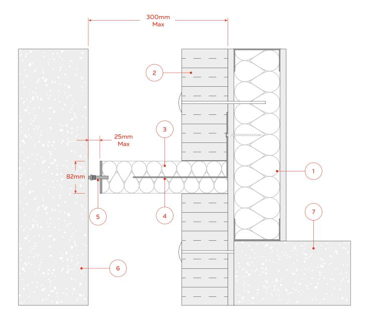
PFC Corofil Open State Barrier COSB 25 (1024) to be installed in line with the product installation instructions See Technical Data Sheet TDSCOSB 25 for full details.
