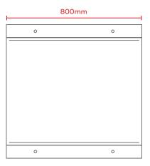
Take a 1 metre strip of PFC Corofil Open State Insert COSI and cut to length, (if the panel is wider than 1 metre, use extra lengths) ensure the total length of the insert is 5mm longer than the cassette panel opening.
