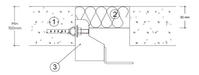
PFC Corofil Cavity Fire Stop CCFS to be installed in line with the product installation instructions. See Technical Data Sheet TDSCCFS for full details.
